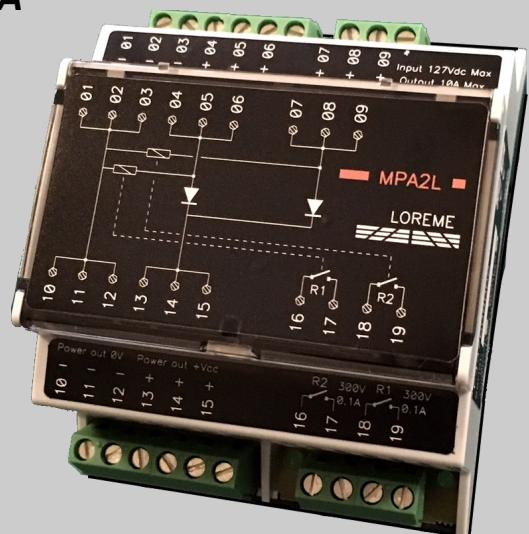
The redundant module provide an effective protection against the power supplies failure.
